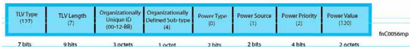
Figure 29-6. Extended Power via MDI TLV
